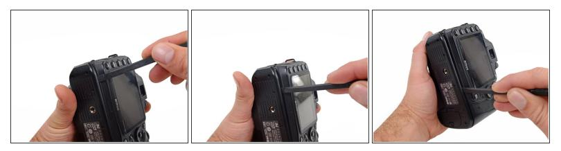
• Using a spudger, separate the bottom panel from the rear case just enough to clear the two clips on the rear casing in the next step.
