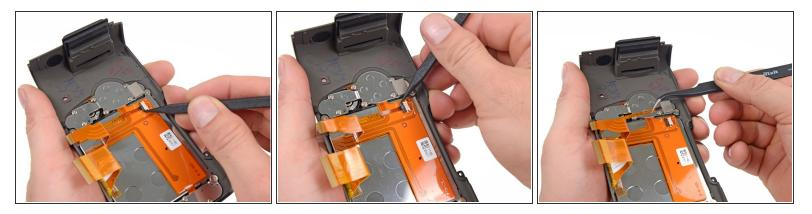
• Using the spudger, rock the connector back and forth to disconnect the cable.
