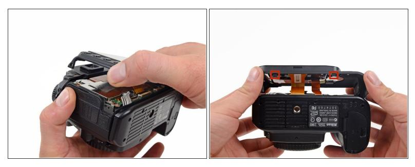
• Lift the rear case off of the back of the camera.
