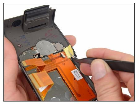
Peel back the yellow tape covering the cable connector on the back of the casing you removed.
