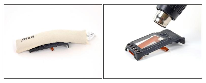
Using either the iOpener or a heat gun, heat the rear LCD glass enough to melt the adhesive holding it on.
