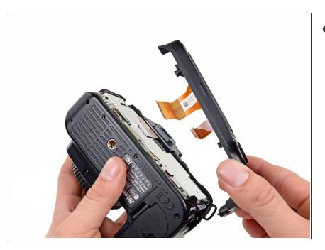
• Separate the rear casing from the camera.
