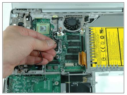
• Deroute the microphone cable from its channel in the metal framework.
