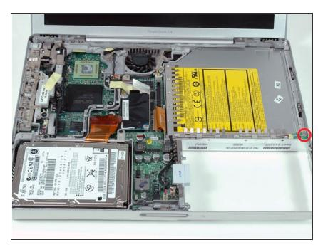
Remove the single Phillips screw securing the hall effect sensor board to the optical drive.
