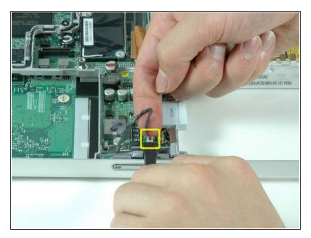
Use a spudger or the tip of your finger to disconnect the sleep light cable from the DC-to-DC board.
