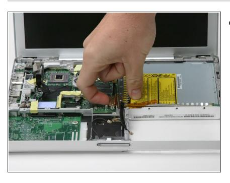
Disconnect the orange optical drive cable from the logic board.
