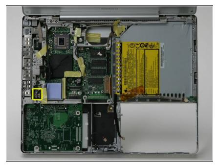
Disconnect the two connectors on the left side of the computer near the ports.
