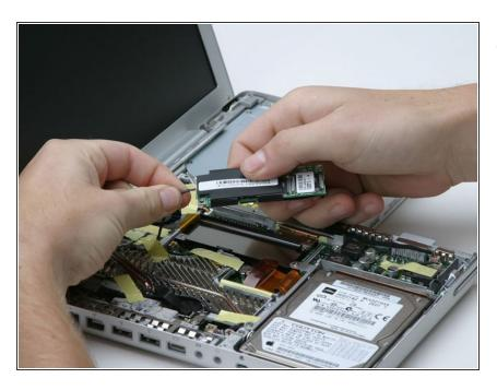
Disconnect the modem cable from the modem.
