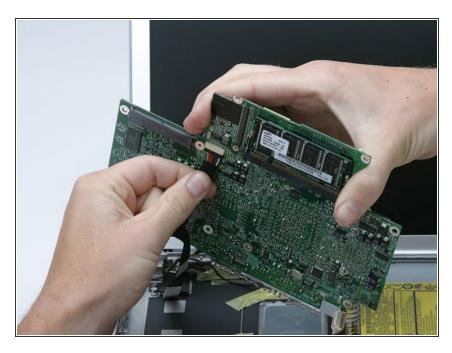
Disconnect the DC-In connector from the underside of the logic board.
