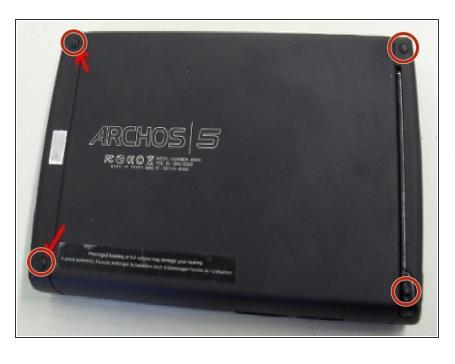
The Back: You can see three rubber pads under which you will find screws. The fourth screw is under the plastic arm. After you removed these four screws, you can easily pop the two plastic pieces on each side of the device.
