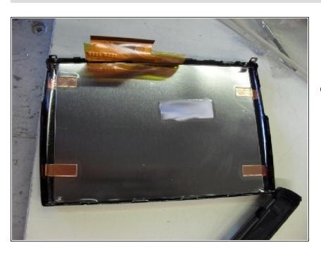
After you remove these eight screws, you will be able to pull the screen away from the rest of the device. Tilt the small plastic strip on the connector to release the wire.
