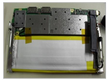
This is the bottom of the motherboard, when the hard drive is disconnected.
