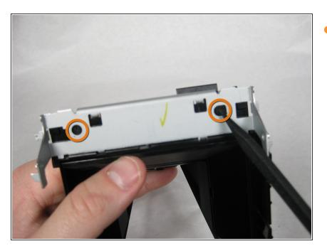
To remove the metal frame, press the two tabs with the spudger and slide it forward.
