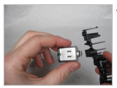
Pull the electric motor straight out of the plastic piece.
