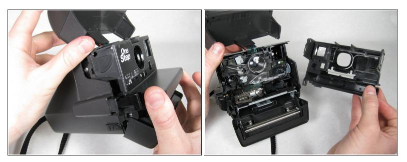
• Once tabs are released, pull face of camera straight out.
