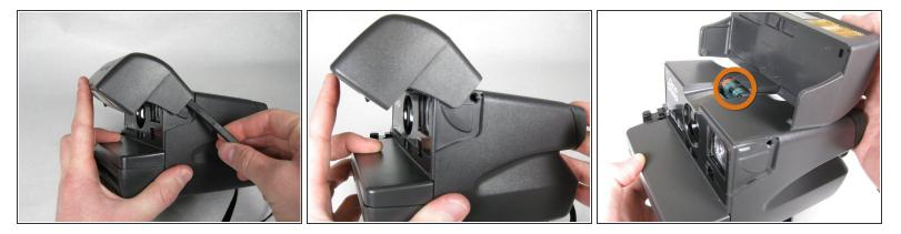
• Separate the flash section of the camera from the main body by unhooking the sides.
