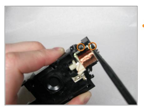
Remove the solenoid from the back of the lens plate by removing the two tabs.
