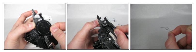
• Lift the large gear away from its pin
