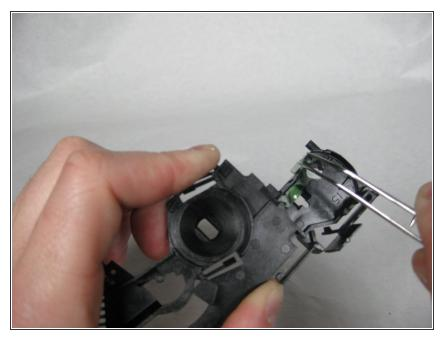
• Remove the clear green prism from the plastic plate.
