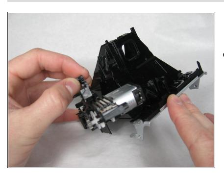
Remove the plastic extension by pulling it from the slot in the rear of the camera.
