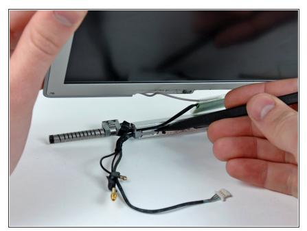
• Use the tip of a spudger to pop the plastic end cap off the left side of the clutch cover.
