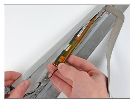
Remove the display inverter assembly from its recess in the clutch cover.
