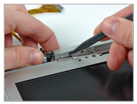
• Use the tip of a spudger to remove the plastic end cap from the right side of the clutch hinges.
