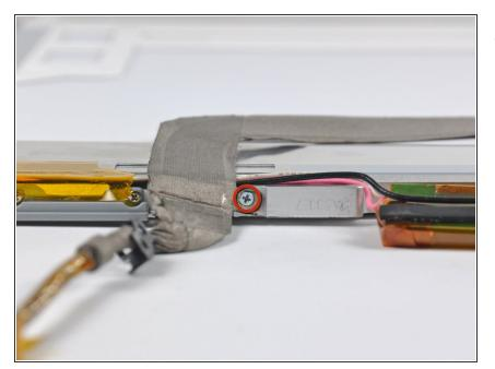
Remove the single 2.5 mm Phillips screw securing the display data cable to the front display bezel.
