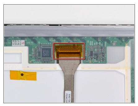
(i) If necessary, remove the piece of tape covering the display data cable connector.
