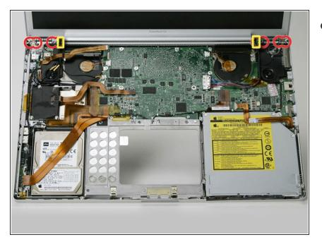
When reassembling the display, check to see that the hinges are seated properly before reinstalling the 8 screws of the two hinges.
