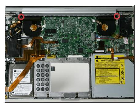
• Remove one T6 Torx screw from the upper, left corner of the left fan, and one from the upper, right corner of the right fan (2 screws total).
