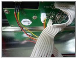
• The small motherboard with the USB and IR receiver PCB.
