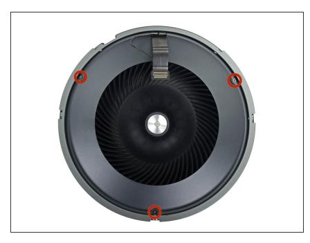
Remove the three 3.7 mm T4 screws securing the fan bezel to the fan assembly.
