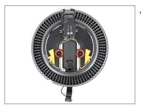
Remove the remaining two 10.4 mm T10 screws securing the fan to the fan assembly.
