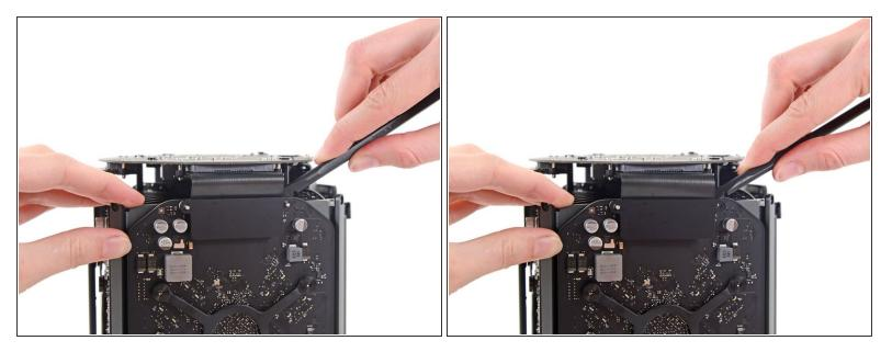
Use the flat end of a spudger and a twisting motion to gently separate one side of the graphics card data connection.
