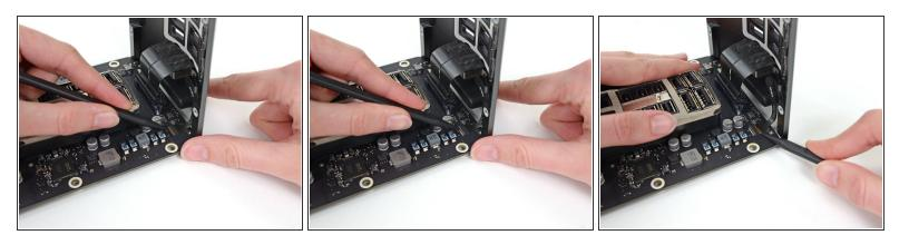
(i) Set the assembly down on a flat surface to access the connectors on the IO board.
