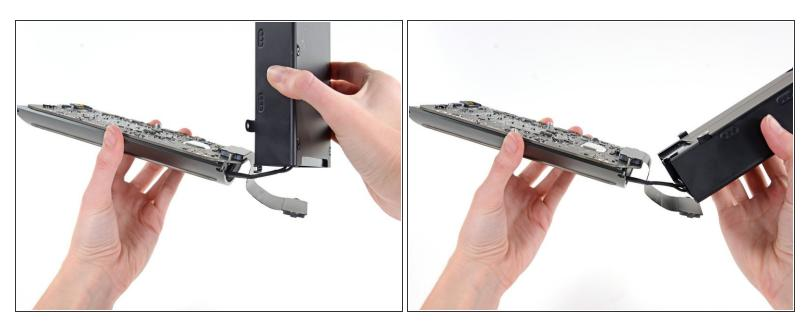
• Flip the power supply back to expose the AC power inlet cable.
