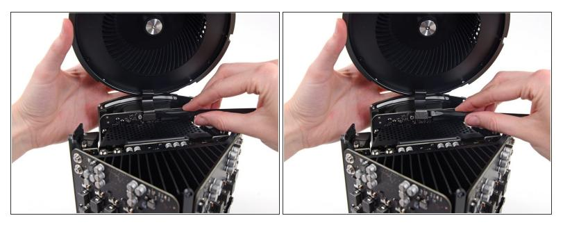
• Use the flat end of a spudger to disconnect the fan assembly ribbon cable from the IO board.
