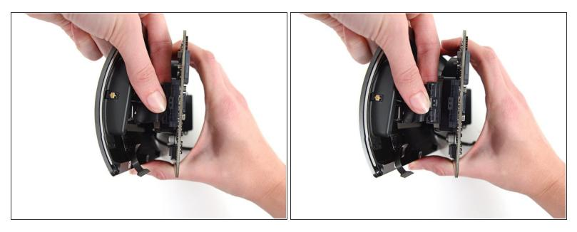
• Squeeze and pull the audio jack ribbon cable connector from the IO board.
