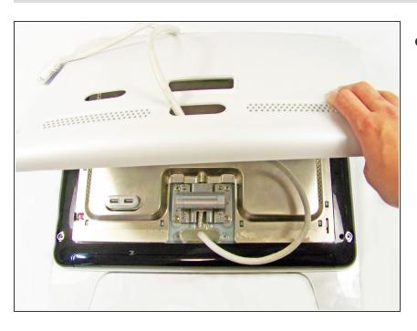
Remove the grey back panel by lifting the bottom and pulling the ADC cable through the hole.
