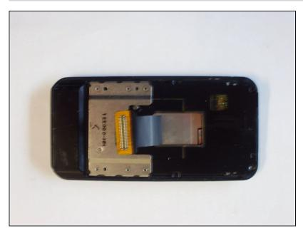
This is how the other half of the phone should look. This part contains the sliding mechanism used to hide the keypad.
