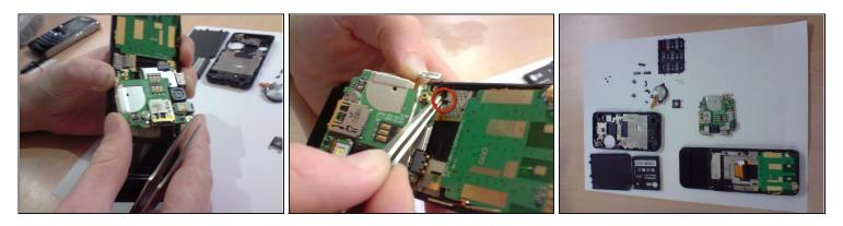
• This shows the detatching of the circuits and all the componets that should be removed.
