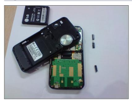
Removing the screws allows you to access the heart of the phone. All the circuitry is housed neatly at the bottom end of the phone.
