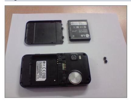
Back panel and battery removed.
