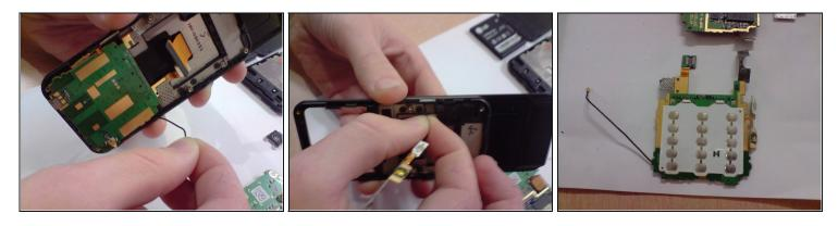
• The key pad is taken out and is an idepandant part. It is easily removed thanks to the snap fits securing it in the phone.
