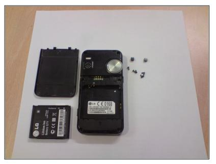
Two screws found under the plastic clips removed as well as another four screws found around the battery.
