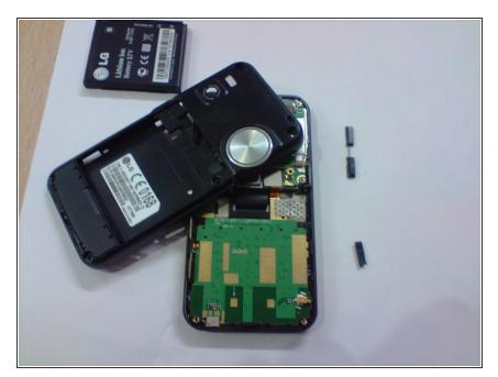
Removing the screws allows you to access the heart of the phone. All the circuitry is housed neatly at the bottom end of the phone.
