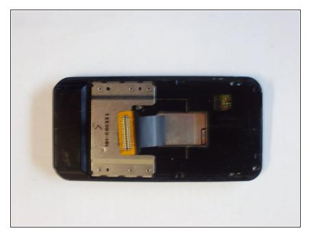
This is how the other half of the phone should look. This part contains the sliding mechanism used to hide the keypad.
