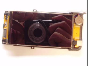
The actual screen will then clip out of the plastic casing protecting it.
