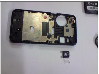
The flash is the next piece to be taken out. It is attatched with some circuit wiring, simply unplug the wiring and the flash pops out of the casing.
