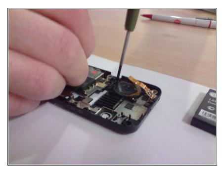
The scrowl wheel is a simple variable resistor, so is easy to detatch, simply unscrew the small screws holding it to the main body of the phone.
