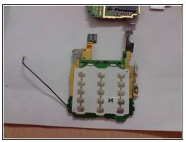
The key pad is taken out and is an idepandant part. It is easily removed thanks to the snap fits securing it in the phone.
