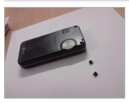
Two plastic clips removed to show the screw heads on the back of the phone.
