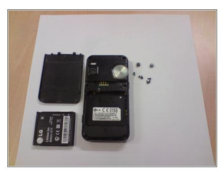
Two screws found under the plastic clips removed as well as another four screws found around the battery.
