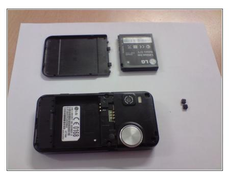
Back panel and battery removed.
