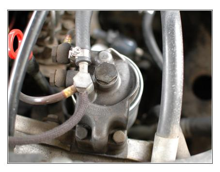
Check for fuel leaks at the spin-on fuel filter housing.
