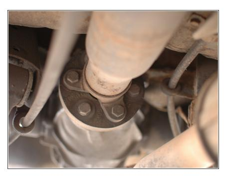
Check the rear flex disc for cracks or other deterioration.
