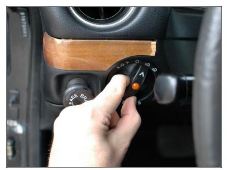
Test the headlight switch. Move it through all positions, from running lights, to head lights, and then back on the other side of the off setting to test the parking lights.
