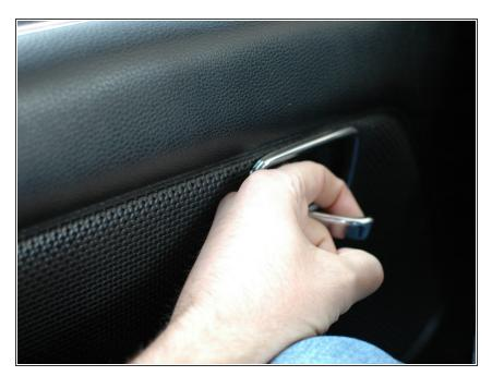
Test all of the door pulls. They should be tight with little to no movement up and down.
