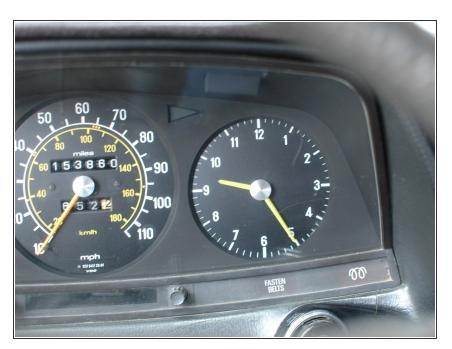
Check that the clock is working. On later models years than the car used in this guide the clock will be smaller and inset beneath the tachometer.
