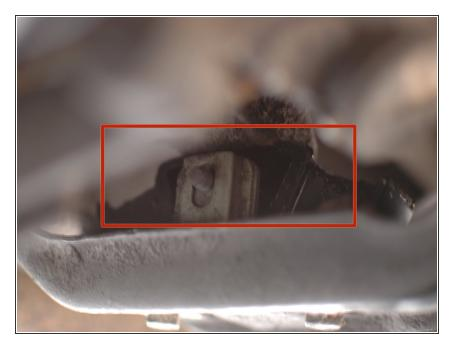
Check the transmission mount for deterioration. It is up inside the cross member just behind the front flex disc. You will have to crane your neck up to see it above the cross member.
