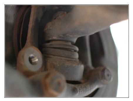
Check the ball joints for cracks or split boots.
