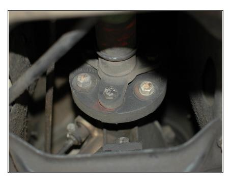
Check the front flex disc for cracks.
