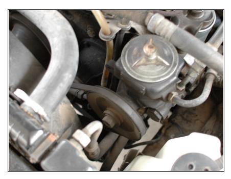
Inspect the power steering, water pump/alternator, and A/C condenser (if applicable) belts for cracks or other signs of wear, and for looseness.
