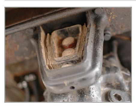
Check the rear differential mount for cracks, dry rotting, etc.
