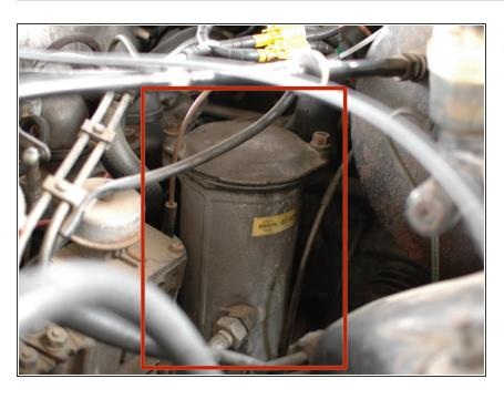
Check the oil filter housing for leaks at the lid seal, as well as at the oil cooler lines and the seal where it attaches to the engine block.
