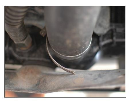
Check the lower hose at the radiator for cracks, stiffness, etc.
