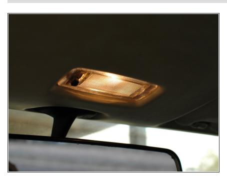
With the front door open the courtesy light should turn on. If it does not, try moving the small black switch on it through its various positions to see if the bulb is burnt out or if another issue may exist such as a bad door switch.
