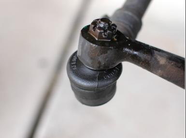
Check all four tie-rod ends for cracked or split boots. Both outer joints shown. Inner joints are at the other end of the tie-rod.
