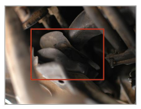
Look up at the end of the engine arms for a second look, from below, at the engine mounts. See that they are still holding the engine well up and away from the sub-frame and also that they do not look dry-rotted or otherwise deteriorated.
