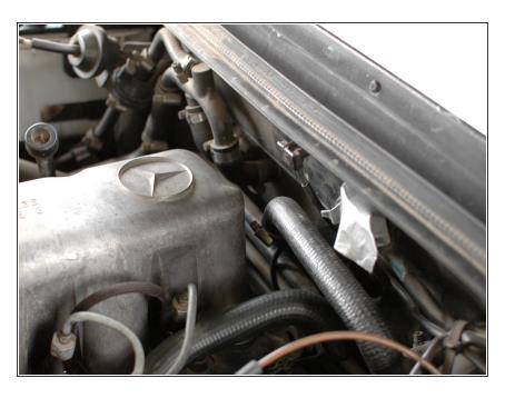
Inspect the various heater hoses for signs of leaking coolant, or for cracks or brittleness in the hoses.
