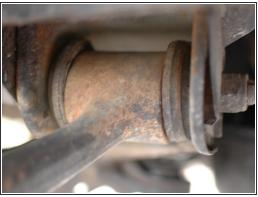
Check the various other rubber boots, bushings, etc. on the front steering and suspension for cracks, splits, dry-rotting, etc.
