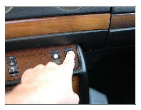
Test the rear window defrost. Leave it on and see that it turns off after the timer period.
