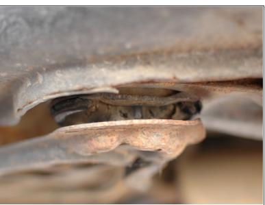
Check the sub-frame mounts for deterioration, this one is collapsed.
