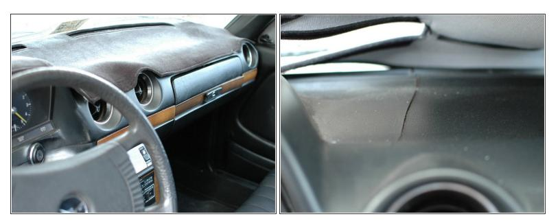
Look at the dash, checking for cracks. If there is a dash cover lift it up as these are usually there to cover up cracks.
