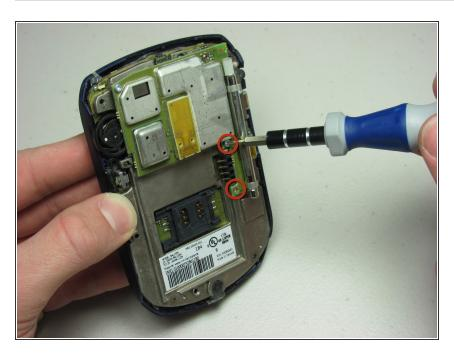
Remove the two T6 screws.
