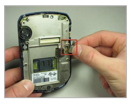
Replace with new vibration motor.
