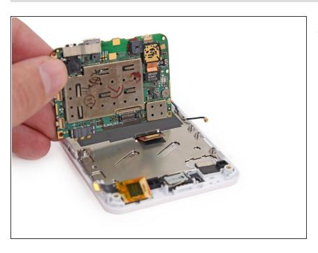
Remove the motherboard from the display assembly.
