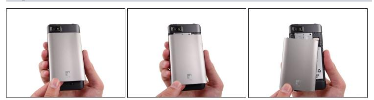
• Slide the back cover down and remove it from the phone.
