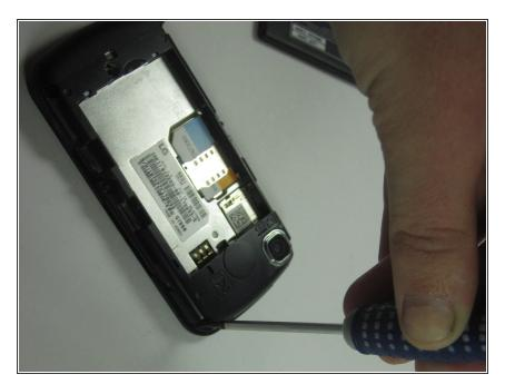
Remove all the screws with a Philips #0 screwdriver
