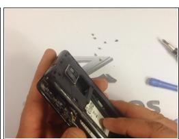
Use a plastic tool to remove the rear housing.
