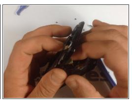
Now, use a suction tool to remove the screen from it's housing. Be careful when doing this, to prevent possible injury.
