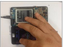
Test the new spare part before reassembling.
