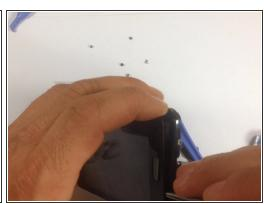
⚠ Be careful with the menu buttons flex cable in the bottom side of the touchscreen. You must release it before separating the digitizer from the frame.
