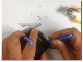
With a cutter, make a room for a plastic tool, then continue with separating the Touchscreen &
