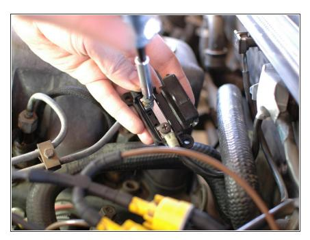
• Replace the fuse box with the new one, and install a new 80 or 50 amp fuse (check to see which fuse to use, depending on year and model). Screw in the two Phillips head screws that hold the glow plugs wires to the fuse and fuse box, and then reattach the new fuse box to the firewall.
