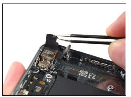
• Using a pair of <u>tweezers</u>, flip the rubber camera cover out of its clip and toward the outside of the rear case.
