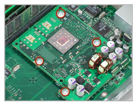
• Remove the four screws holding the CPU to the motherboard.
