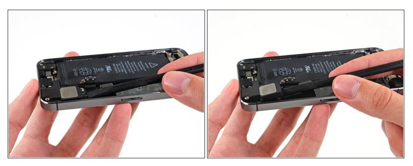
Use the flat end of a spudger to gently lift the speaker from the rear case.
