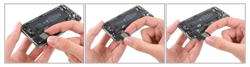
(i) The speaker has a small peg that slides into a slot beneath the home button cable socket.
