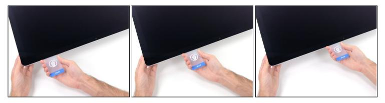
$\triangle$  Be sure to stop cutting before the iSight camera in this step, or you may damage it.
