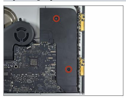
Remove two 10.0 mm T10 screws.
