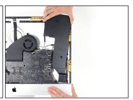
• Lift the speaker straight up and remove it from the iMac.
