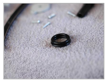
For reference, you can see a comparison here. The original MityVac o-ring is on top, the new oring is below. The new o-ring is slightly thicker and, as long as it fits in the body of the pump without binding, it should provide a better and longer lasting seal.
