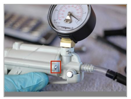
Remove the two screws on the front of the pump body. A #0 screw driver works well. The front cover of the pump can then be gently pulled forward away from the pump body.
