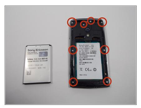
Start by having the screen of the phone facing downwards and remove the battery. Remove eight 5mm screws located as shown with a T-6 bit.
