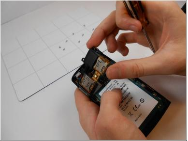
The audio jack can only be accessed if the internal casing is removed. To remove this, apply
