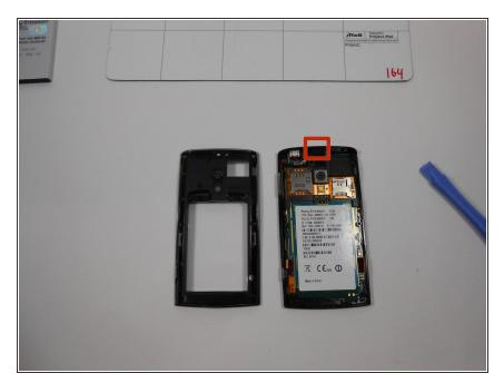
Once the clips are undone the back casing should dislocate and reveal the internal components of the phone. Audio jack location is identified on the image.
