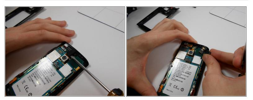
Audio Jack is located and easily removed. New component can be inserted.
