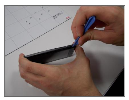
Using a case opener, start on the bottom right side of the phone and undo clips located at the interior sides. Repeat this step for the left side.
