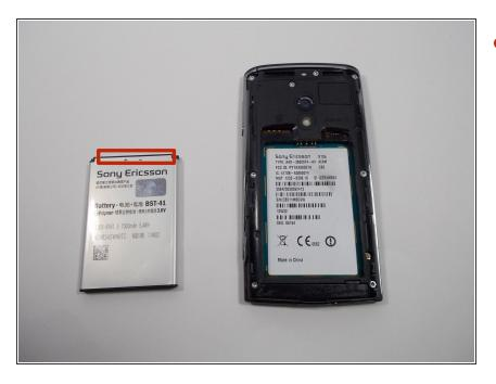
Once battery is removed check the water damage sticker. Red circles on the sticker implies battery damage, and replacement is necessary.
