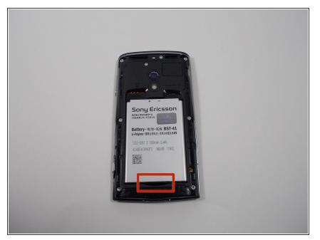
Flip phone so the screen is facing downward and remove the back casing. Locate marker for easy power source removal.
