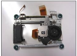
• Remove any tape fastening the cables to the motherboard and gently lift and remove the optical drive.
