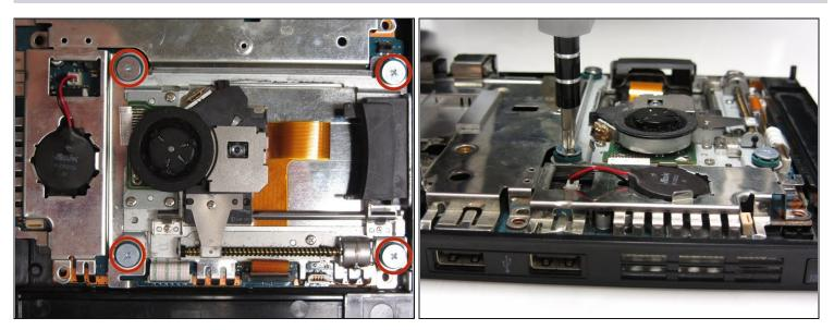
Remove the four 4.0 mm screws using a #1 Phillips screwdriver.
