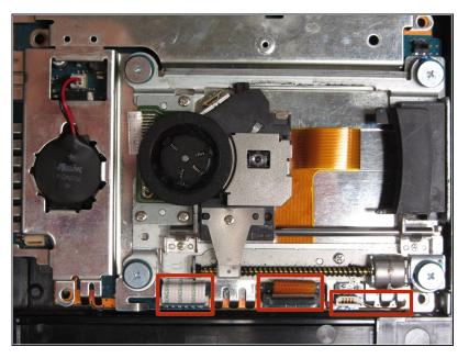
Locate the three ribbon cables connecting the optical drive to the motherboard.
