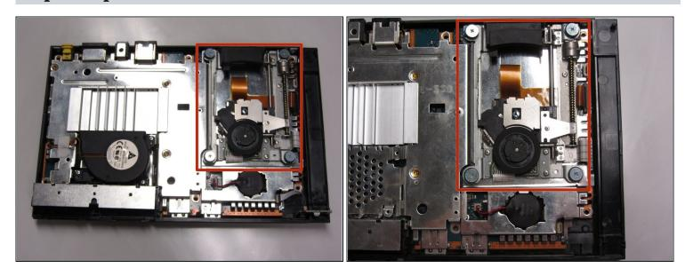
• Locate the optical drive which occupies most of the space on the right side of the unit. It can be identified by the four screws with wide-diameter heads fastening the optical drive to the motherboard.
