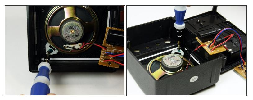
• Remove the two 7/16" screws located in the bottom left and top right corners with a phillips head screw driver. After removing the screws, the metal clips will need to be removed as well.
