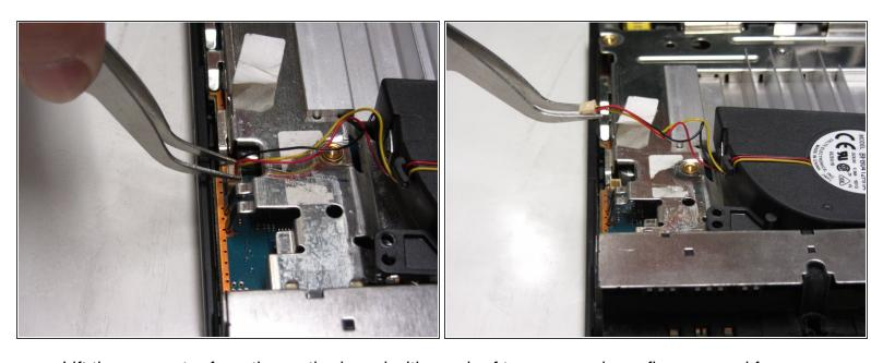
Lift the connector from the motherboard with a pair of tweezers using a firm, upward force.
