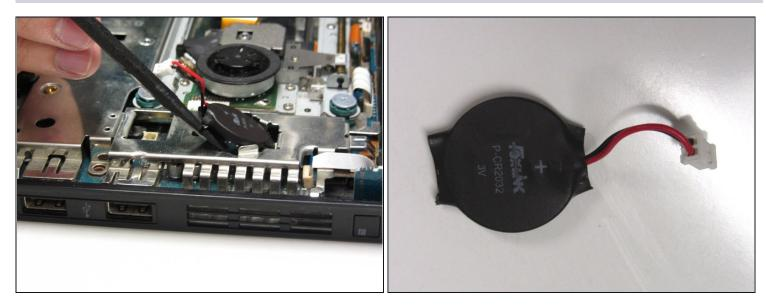
• Gently lift and remove the battery from its compartment using a spudger.
