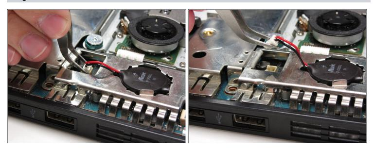
• Lift the connector from the motherboard with a pair of <u>tweezers</u> using a firm, upward force.
