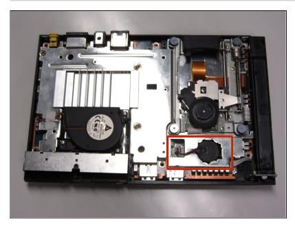
Locate the clock battery at the front, right section of the unit.
