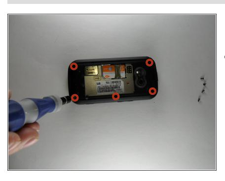
Remove 5 screws, 1 from each corner of the phone and 1 from the center-right of the phone.
