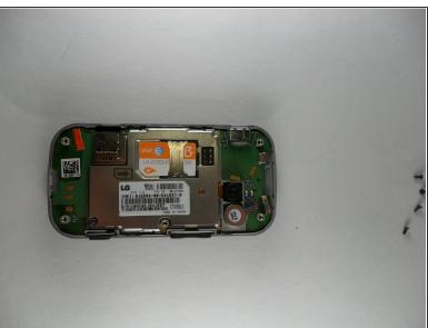
Now pull off the rear casing, using an opening tool. \*\*Buttons for volume and pictures may fall out\*\*
