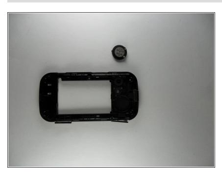
Replace the broken speaker with a new one (make sure to line up the tab with the groove). Push firmly into place. Follow reverse instructions to put the rear casing and back cover on.
