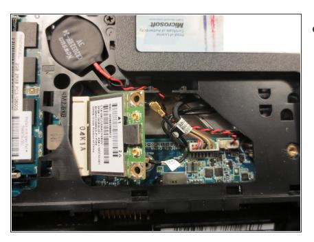
• Lift up on the WLAN module to fortyfive degrees, and gently pull it out.
