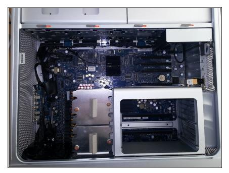
You want to pull off the grey fanassembly on the left (already gone in the pic), for that you have to unscrew 4 Screws in the memorycompartment on the right, slide that to the right and take out the middle cover for the processors
