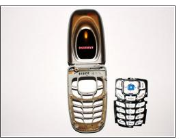
Remove the keypad from the body by grasping the white rubbery pad and lifting it off the phone.
