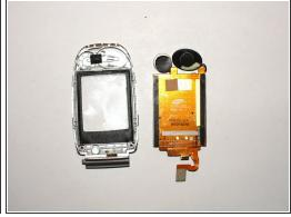
Next use a plastic opening tool to pry the screen from the cell phone cover.
