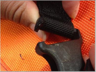
• Using scissors (preferably industrial scissors), cut buckle off and remove buckle from fabric loop.
