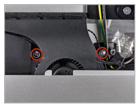
Remove the two 13 mm T10 Torx screws securing the CPU fan to the outer case.
