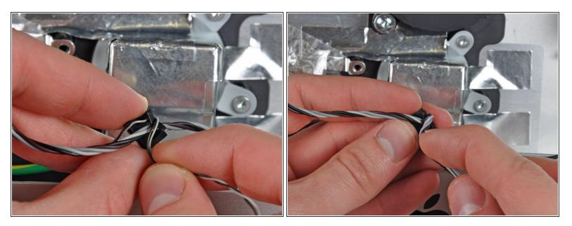
Carefully remove the left speaker and ambient temperature sensor cables from the CPU fan cable retainer.
