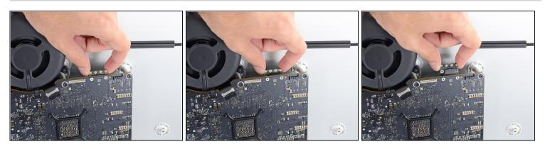
To avoid damaging its socket, do not push the end of the AirPort/Bluetooth Card away from the logic board excessively.
