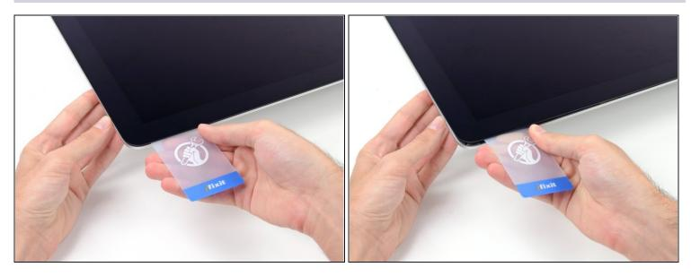
• Gently twist the plastic card to open the space between the display and frame, and cut any remaining adhesive near the corner.
