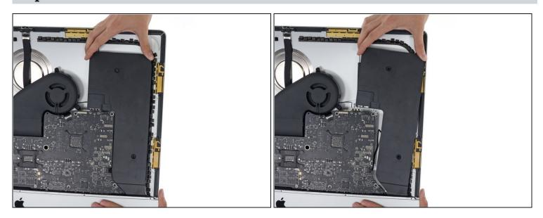
• Gently rock the right speaker slightly to the right, to allow access to its cable's connection on the logic board.
