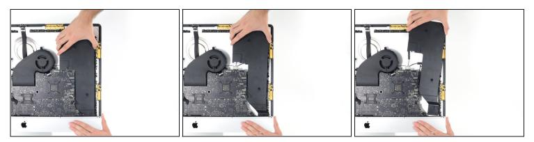
• Lift the speaker straight up and remove it from the iMac.
