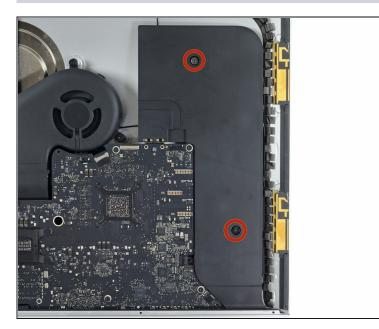
• Remove two 10.0 mm T10 screws.
