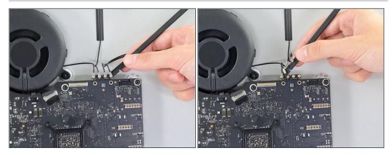
• Use the flat end of a spudger to disconnect each of the four antenna connectors from the AirPort/Bluetooth card.
