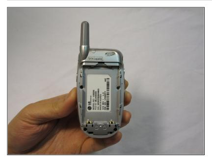
Orient the phone as shown with the battery already removed.
