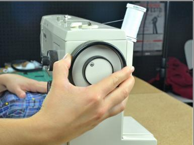
Use the balance wheel to sink the needle into the fabric.
