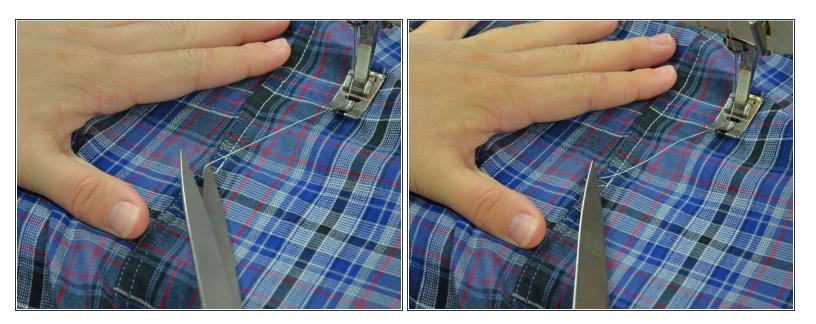
After you've completely sewn over the torn seam, clip the threads and free the garment from the machine.
