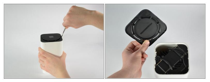
• Using a metal spudger, gently pry the cover off the bottom of the device.
