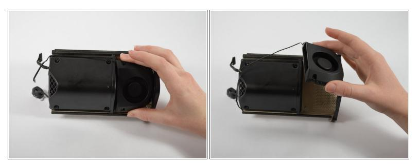
• Remove the fan from the device.
