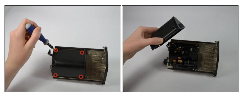
• Remove the four 10.35 mm Torx T8 screws on the black plastic shell.
