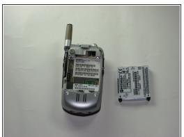
Remove the battery from the phone by gently pulling upward on the battery with your fingers.
