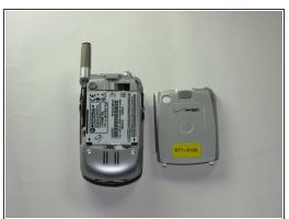
Press down on the back button while pulling away from the body of the phone to release the back cover.
