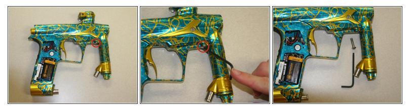
• Use 1/8" allen wrench to remove screw behind regulator.
