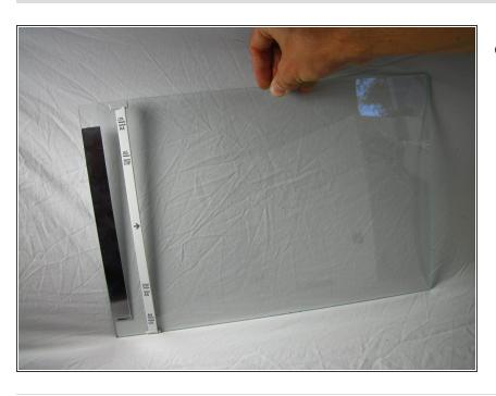
Take out the damaged glass and fit the replacement glass to the printer according to the picture.
