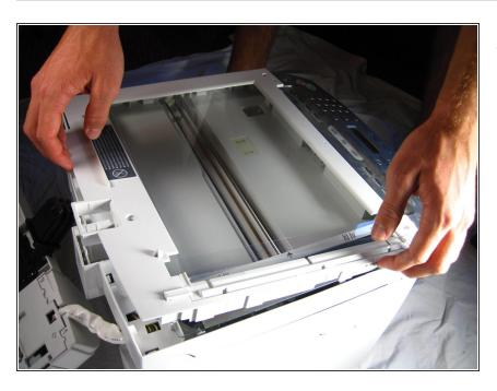
Gently, pry off the top plate, starting from the back of the printer.
