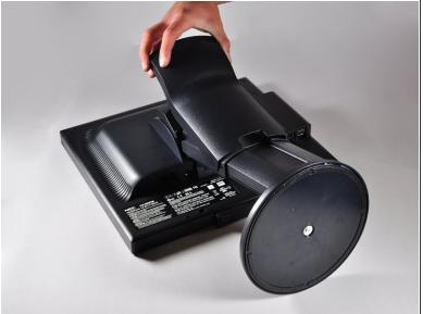
Firmly remove the back panel of the stand by pulling it up and away from the monitor.
