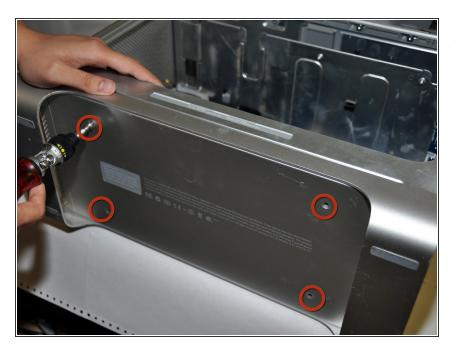
Remove the 4 Philips screws on the underside of the computer case.
