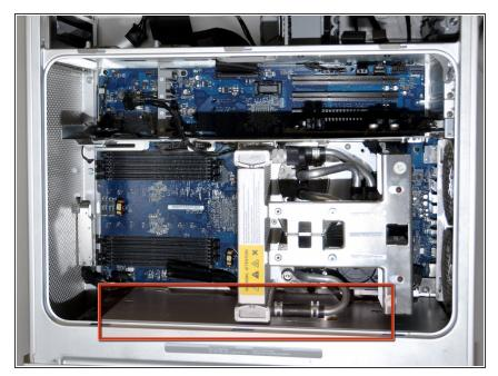
Locate the power supply in the Apple G5 computer. It is located under the metal plate at the bottom of the computer case.
