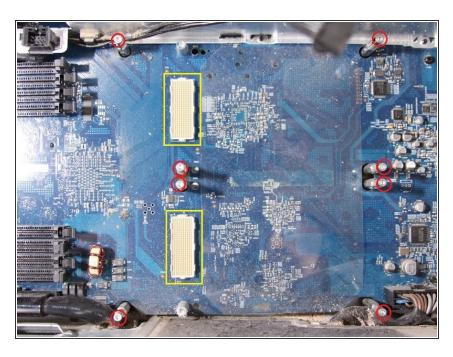
NOTE: Here are the standoffs without the cooling unit installed to make it easier to understand where
