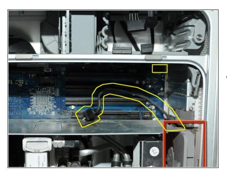
Unplug the fan's power cable from the upper rightmost corner of the motherboard (connection J45). If there is a video card in place, carefully pull the cable plug down between the back edge of the video card and the motherboard. Note, the photo shows the unplugged cable and the area it plugs into outlined in yellow. No video card is shown in this photo.
