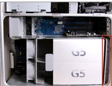
The cooling fan unit is located on the bottom right of the Apple G5 Desktop.
