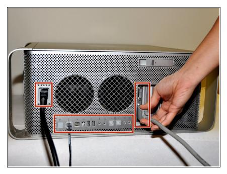
Remove all the cables, including the power cables before opening the unit.
