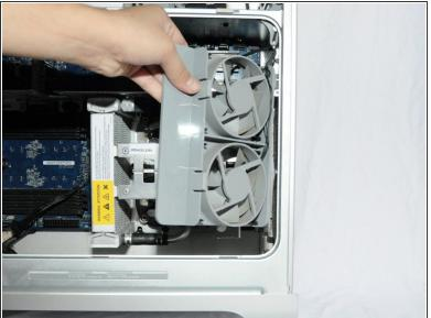
After the latches are out, pull the fan out.
