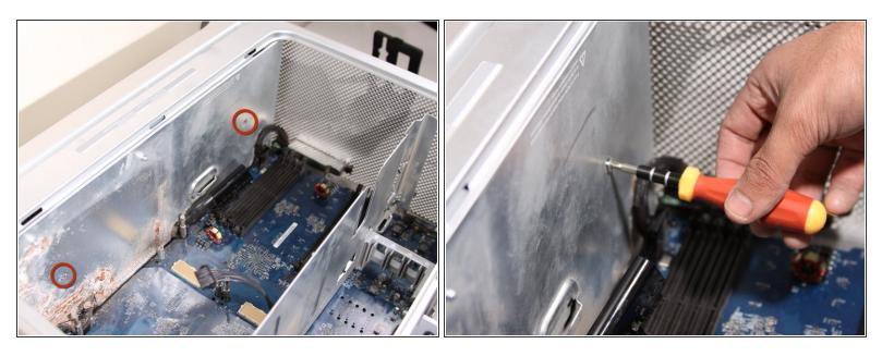
Remove the 2 Philips screws holding the power supply cover on.
