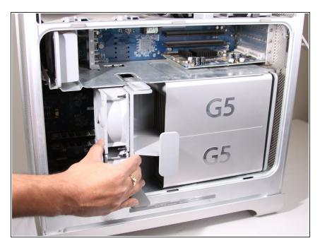
Pull the fan assembly out; it should slide out easily.
