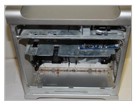
The bottom of the computer should look like this when removal of the power supply is complete. To reassemble your device, follow these instructions in reverse order.
