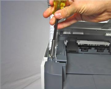
Locate and remove the two 10mm side screws. There is one on each side.
