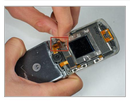
Flip over small hinge that covers the camera ribbon connection.
