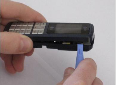
Run the tool along the seam to release all the tabs.
