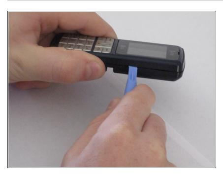
Insert a plastic opening tool in the seam.
