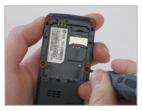
Remove all four screws on the back of the phone using a Phillips #00 screwdriver.
