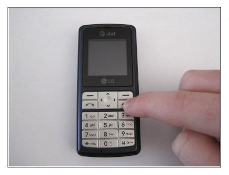
Power down the cell phone by pressing and holding down the red "end call" button.
