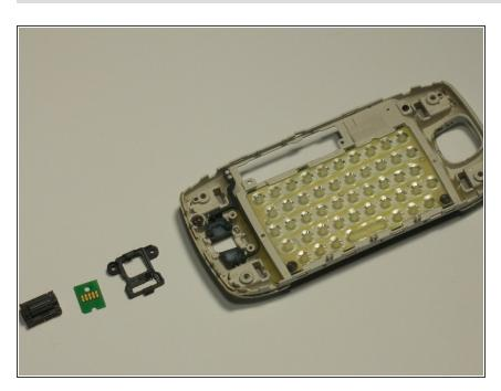
The thumbwheel and casing will be loose, gently remove it.
