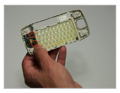
Remove 2 screws using the Torx 6 screwdriver.
